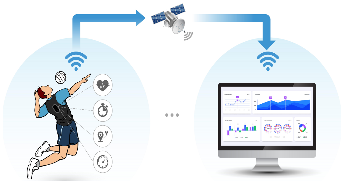
FIGURE 2. Illustration of the wearable inertial sensor device and data collection process.
